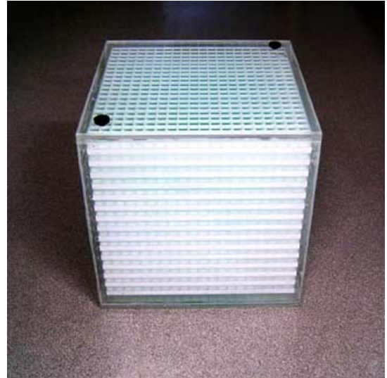
Fig. (4). A photograph of a 3D phantom based on a new design approach using a concept that a point in 3D can be defined by the intercepting point of the three orthogonal planes.
